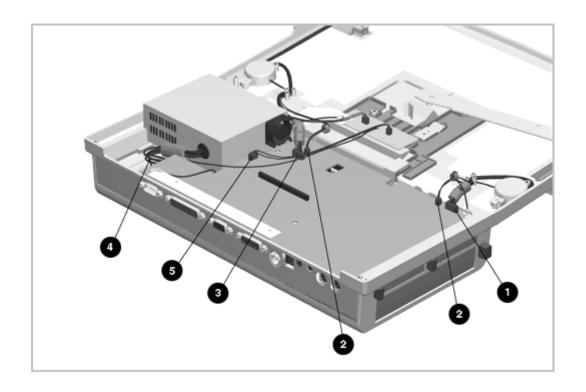
Figure 6-15. Disconnecting and Removing the Main Board Cables
